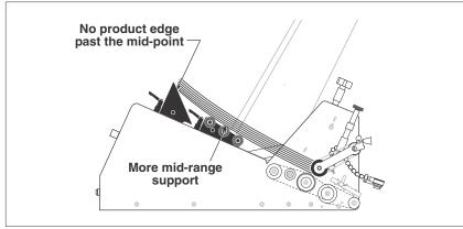
Figure 6-5. Separate Triangle and Low-Profile Wedge Setup
