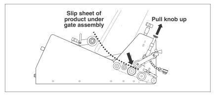
Figure 2-1. Lifting Gate Assembly Upward to Insert Material
