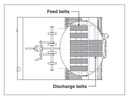
Figure 5-1. Inspecting Feed and Discharge Belts
