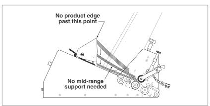
Figure 6-1. Load Compensating Wedge Setup
