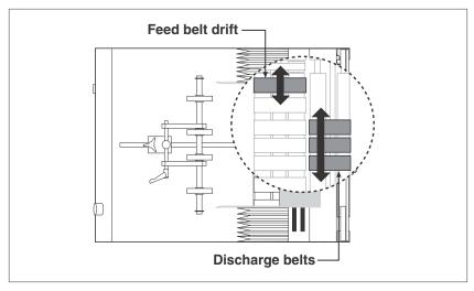
Figure 5-3. Ensuring Proper Feed Belt Tracking
