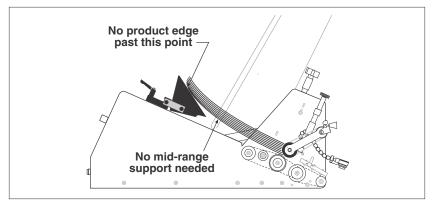
Figure 6-3. Extended Narrow Wedge Setup
