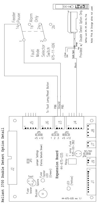
When in Alarm Only, feeder will reset Feach the sensor what a double is by placing two pieces of material between the sensing elements at its least The Double Detect sensor has an NPN sinking output. Set the sensor switches to: Lock Off, Off, Dark On, Fine. densest point (avoid print, etc.) then press and hold the set button until the yellow LED blinks. Put the Fault Mode Switch in the Stop position and force a double to verify proper setup. on the next valid trigger. Notes:
