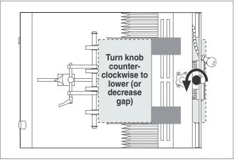
Figure 2-3. Adjusting Gate Assembly for Correct Gap
