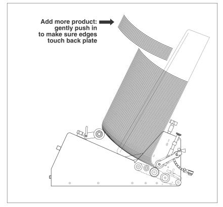
Figure 3-3. Adding More Material to Hopper
