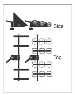
When to use: If moving separate triangle wedge assembly back from the gate assembly, bottom of stack still touches table top, you need mid-range support.
