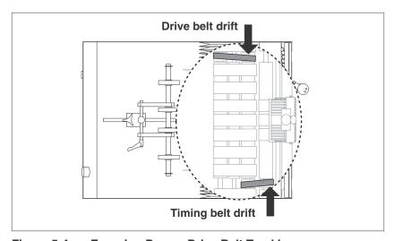
Figure 5-4. Ensuring Proper Drive Belt Tracking
