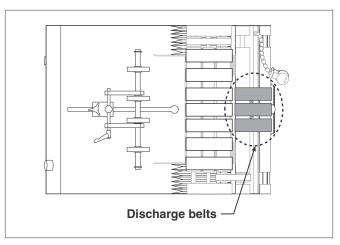
Figure 5-12. Cleaning Discharge Belts
