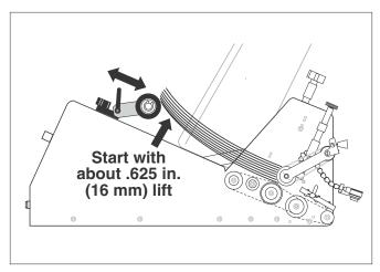
Loosen locking lever to swivel forward or backward
