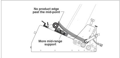
Figure 6-6. Separate Articulating Roller and Low-Profile Wedge Setup
