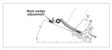
Figure 2-10. Positioning Material Prior to Loosening Back Wedge
