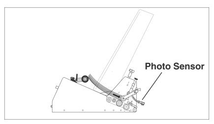
Figure 2-15. Adjusting Photo Sensor for Perpendicular Position
