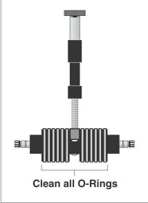
Figure 5-14. Standard O-Ring Gate
