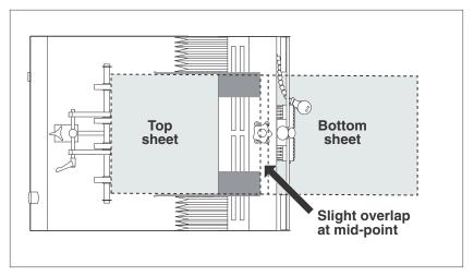
Figure 2-16. Optimum Overlap and Separation of Material
