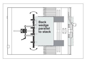
Figure 2-13. Adjusting Back Wedge for Parallel
