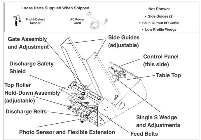
Figure 1-1. Main Assemblies of the Reliant 3700 Universal Friction Feeder
