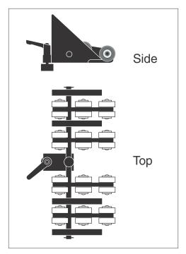
When to use: For thin material with minimal body, thus requiring minimal mid-range support.
