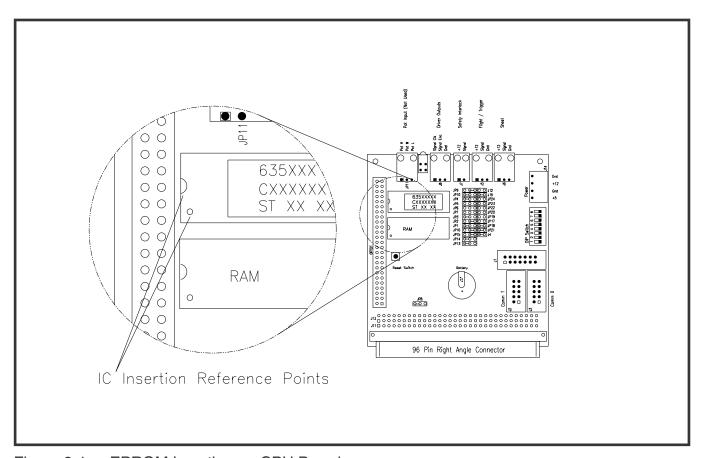
Figure 8-1. EPROM Location on CPU Board
