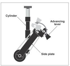
Figure 5-8. Advancing O-Ring Gate
