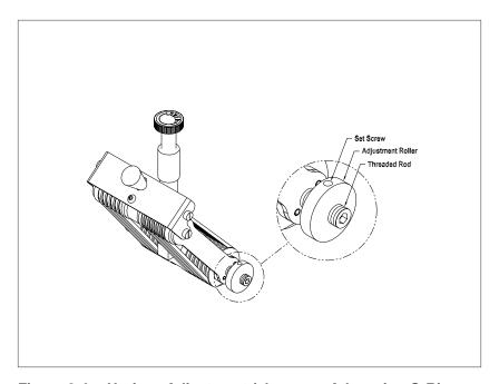
Figure 2-4. Horizon Adjustment (shown on Advancing O-Ring Gate)
