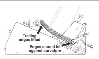
Figure 3-2. Leading Edges Against Gate Bracket Assembly and Side Guides
