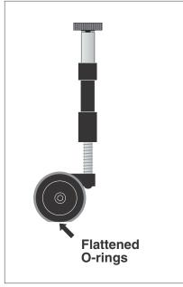
Figure 5-6. Standard O-Ring Gate
