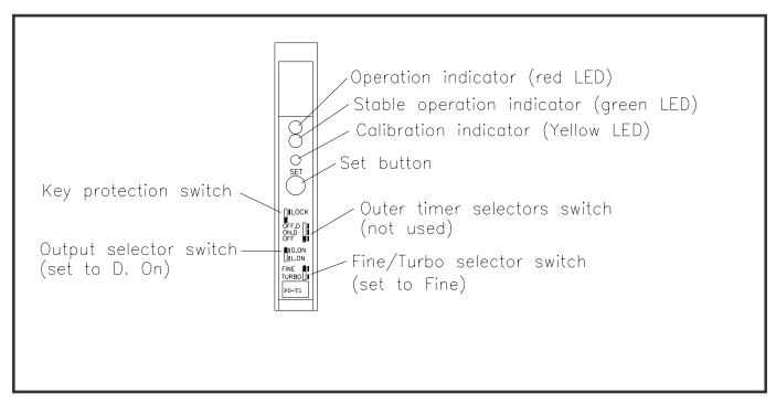
Figure 8-4. Sensor Components and Switch Settings
