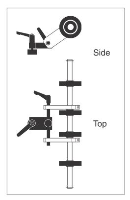
**When to use:** Effective for very thick and/or ridged material. Due to characteristics of material, no mid-range support is required.
