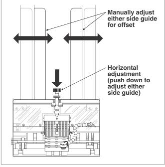
Figure 2-6. Horizontal Adjustment of Side Guides
