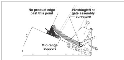
Figure 6-4. Combination Triangle/Low-Profile Wedge Setup
