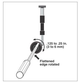
Figure 5-9. Standard O-Ring Gate
