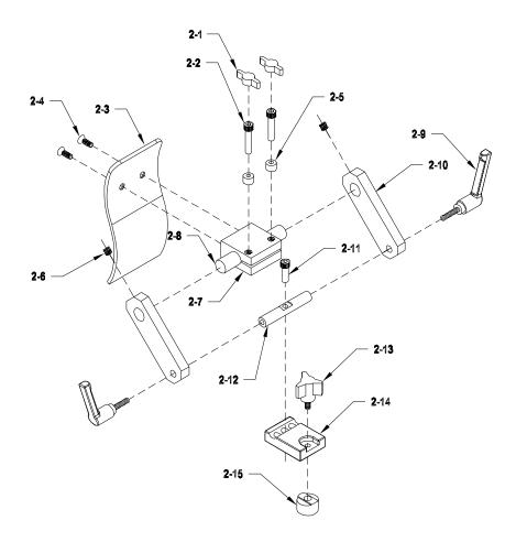
Diagram 2 Single S Wedge Assembly #63311026 REV A
