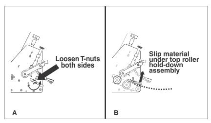
Figure 2-14. Adjusting Top Roller Hold-Down Assembly
