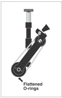
Figure 5-5. Advancing O-Ring Gate
