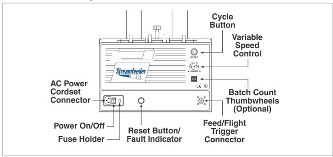
Figure 1-2. Control Panel Components
